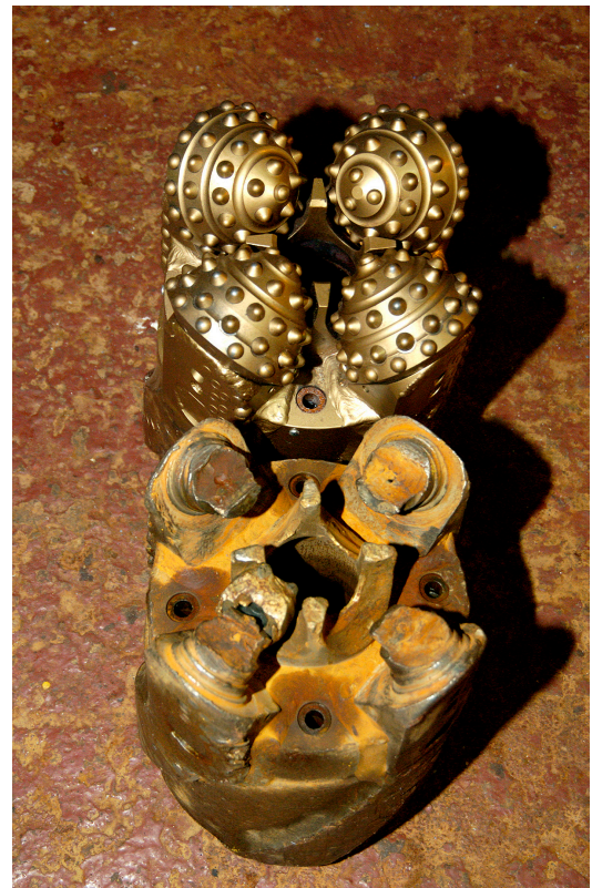
Rotary core drill bits before and after drilling, Expedition 312.
