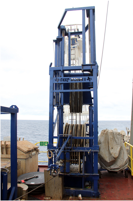
Wireline heave compensator framework.
