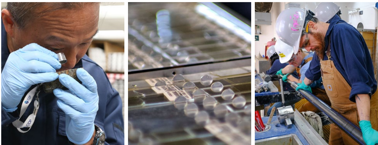
From left: Taking a closer look at a rock sample. Smear slides neatly arranged in slide trays. Closing voids caused by gas expansion.
