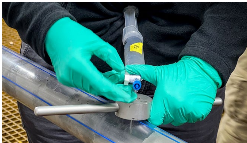
From left: Examining foraminifera through a stereoscope. Collecting a gas sample through the core liner on the catwalk.
