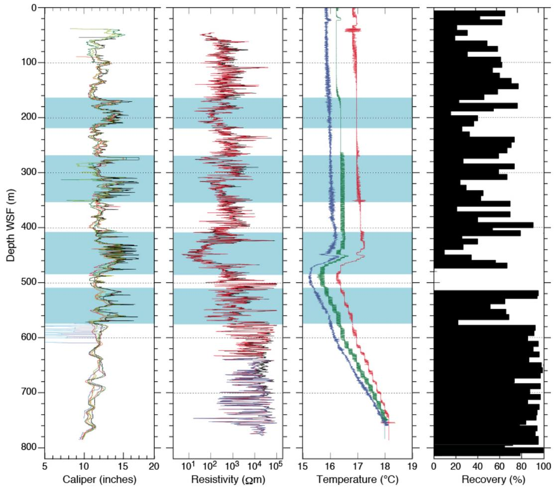
**Figure A1.** Downhole logs of Caliper, Resistivity, and Temperature, as well as Core Recovery (%) for hole U1473A
