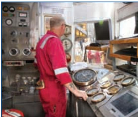
Command center for drilling operations: "the driller's shack"
