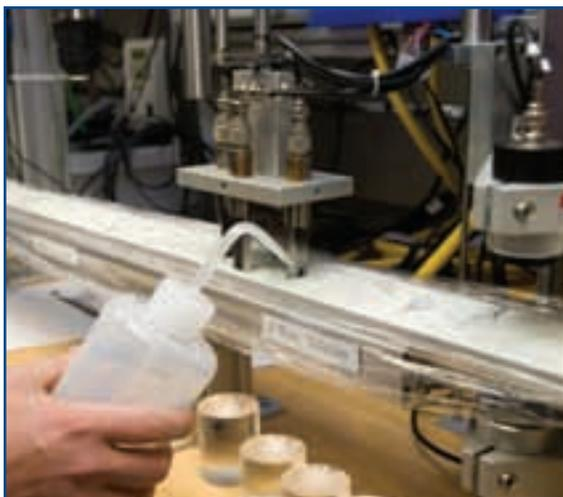
*P-wave velocity measured with the Gantry System*
