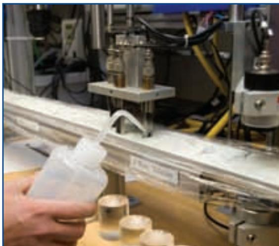
*P-wave velocity measured with the Gantry System*
