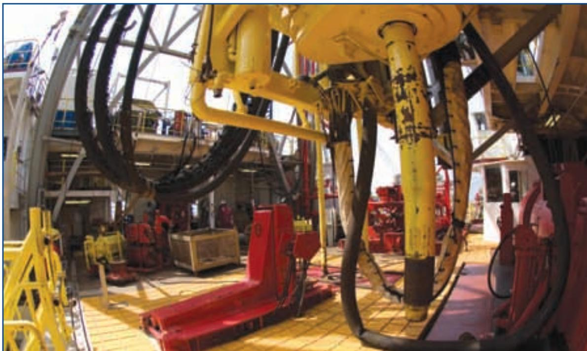
*Passive heave compensator from the rig floor*
