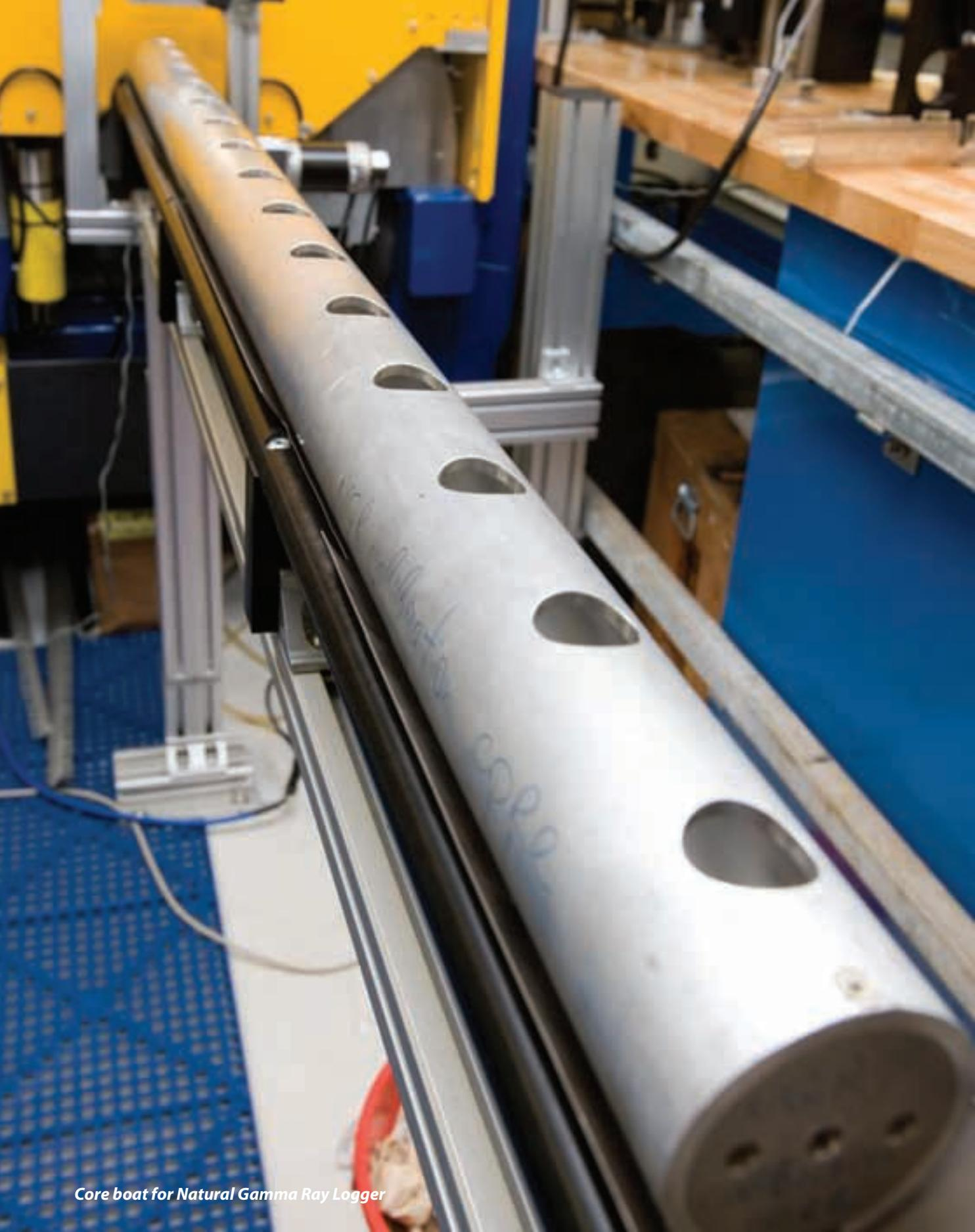
*Core boat for Natural Gamma Ray Logger*
