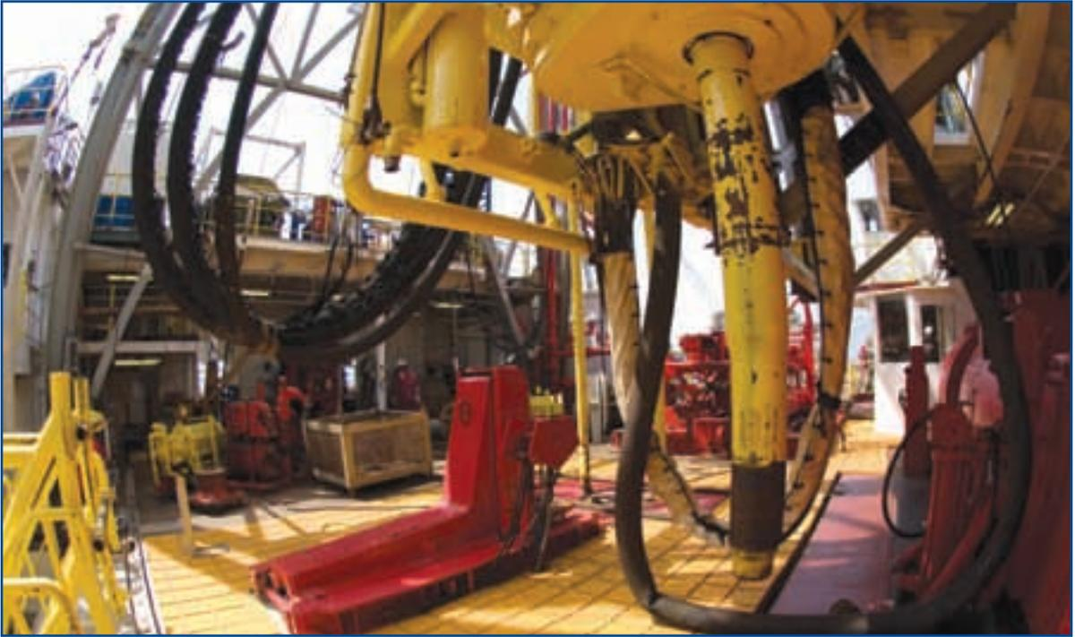
*Passive heave compensator from the rig floor*
