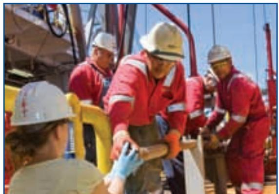
Receiving core from the rig floor
